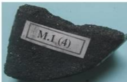
MẪU 1 (4) 40% than mỡ Sơn La + 60% than gầy Hòa Bình
