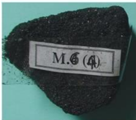
MẪU 6 (4) 50% than mỡ Sơn La + 50% than gầy Hòa Bình
